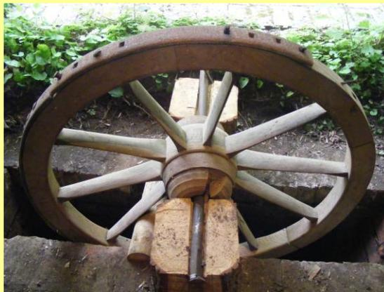
**Wheel in the Straking Pit with loosely attached strakes**
