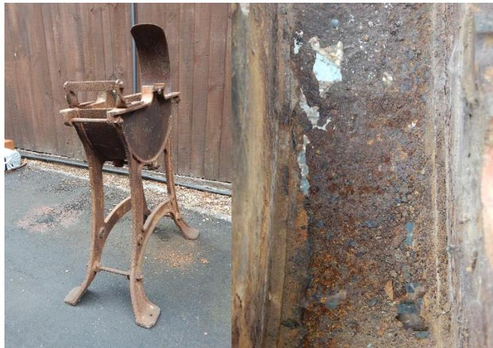
The main body of the grinder is comprised of two cast iron side plates and a sheet steel panel between the two which then forms the water trough.
