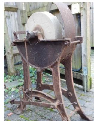
The stone we have is 18" diameter and the grinder would have cost 27s 6d (137.5 p) when new. At the turn of the century this was an expensive item. It is in need of some renovation including repairing the stone itself but no work has been done to renovate it, at present, due to restrictions on movement etc. but our plan is to repair and renovate so that it can be used again.
