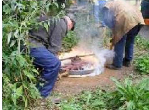
The hot tyre was placed over the wooden wheel and tapped into place. Due to the high temperature of the tyre the wood starts to burn. Once in place the tyre is cooled with a large quantity of cold water.
